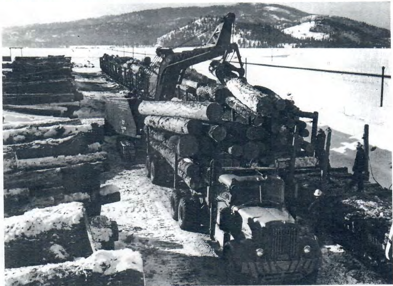
The Anaconda Copper Mining Company built a major log loading facility at Clearwater Junction. This scene is from 1948. Trucks hauled logs from the surrounding area to Clearwater where they were loaded on the Milwaukee spur line for transport down the Blackfoot Canyon to the Bonner mill.
