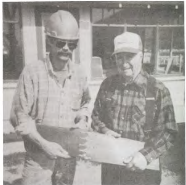
Mike (Woody) Woodworth and Duke Doucett display conveyor belt splicing with leather lace.
